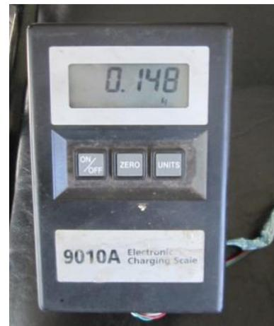
**Gambar 5.** Disply Electronic Charging Scale
